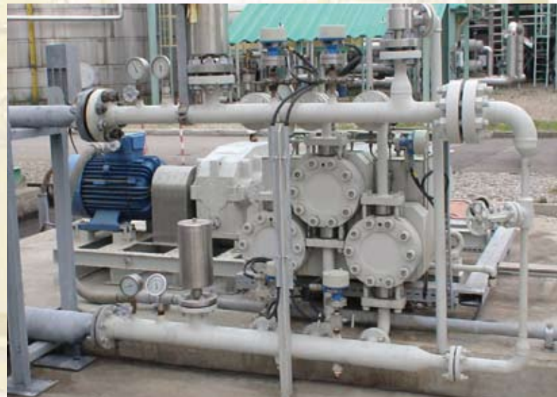
Titano 31.30 m Triplex Diaphragm Pump for Water Reinjection in an oil field
