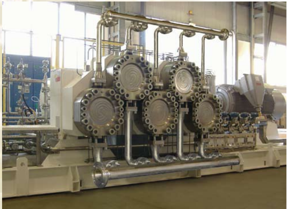
PQO 160 m Quintuplex Diaphragm Pump for Sour Water Injection in an oil field
